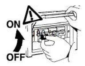
**Note:** To take off the lamp, firstly turn off the power, remove the front cover, then loosen the ears, make it toward the inner side, Be careful not to use too much force, in case damage the ceiling or pulled wires and drives.
