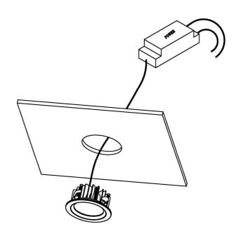
10. After pushing the driver inside the ceiling, First counterclockwise to loosen the ears, then clockwise to tighten the ears onto the ceiling,
